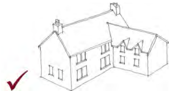
Simple pitched roof forms create uncomplicated roofscape on extension to rear elevation
