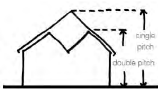
Above: illustration showing that using a double pitch reduces the overall building height
