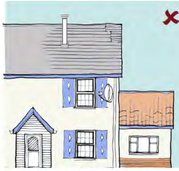
Example 2: Unsympathetic repairs and alterations
