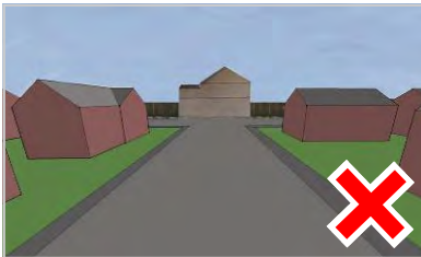
Blank side elevation of dwellings
