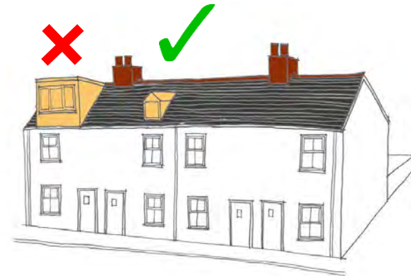
Fig F.4 Dormers should reflect the symmetry and size of other windows on a house. Front dormers are discouraged if not a feature of the street
