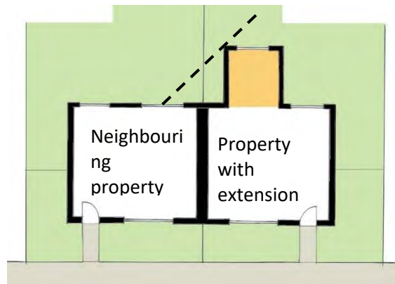
Fig B.3 The 45 degree rule helps prevent overshadowing
