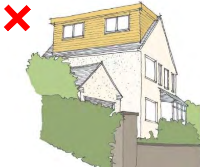
Fig F.6 A large, poorly designed dormer extension can dominate a house and the streetscene
