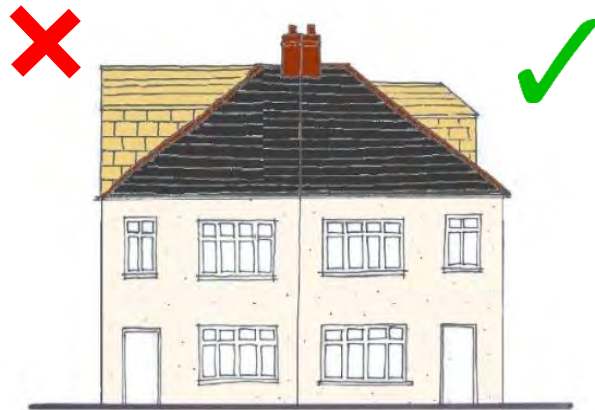
Fig F.5 The dormer on the right is appropriately subservient within the roof plane and the hipped roof design mirrors the hipped roof of the original house
