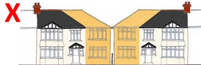
Fig B.2 Over-scaled extensions that result in the terracing effect (above) and well-proportioned side extensions that retain a 1m gap (below)
