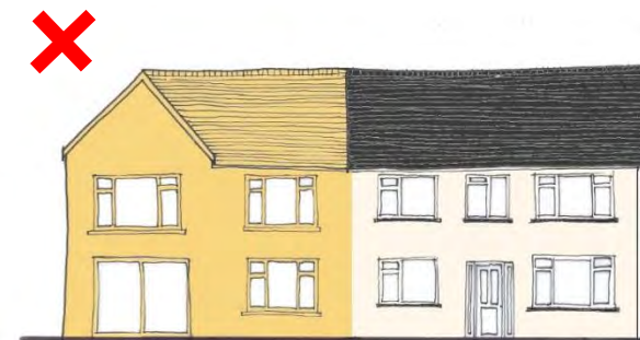
Fig A.2 A poorly designed side extension that competes with the scale and form of the original house
