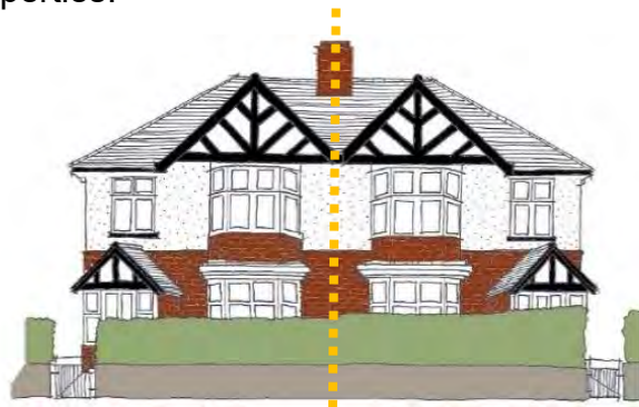
Fig B.1 Semi-detached properties often have a very strong symmetrical relationship which should be retained
