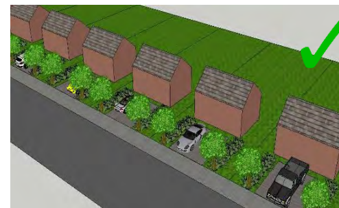
Fig 4.11 Parking should be combined with planting and SuDS features, where possible
