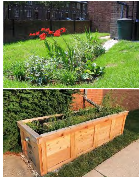
Fig 3.3 Rain gardens can be surface level and include water butts (top) or provided as planter boxes (bottom)
