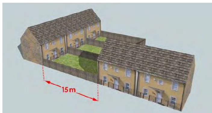
Fig 3.5 A minimum separation distance of 15m is required between a blank two storey wall and existing habitable room window
