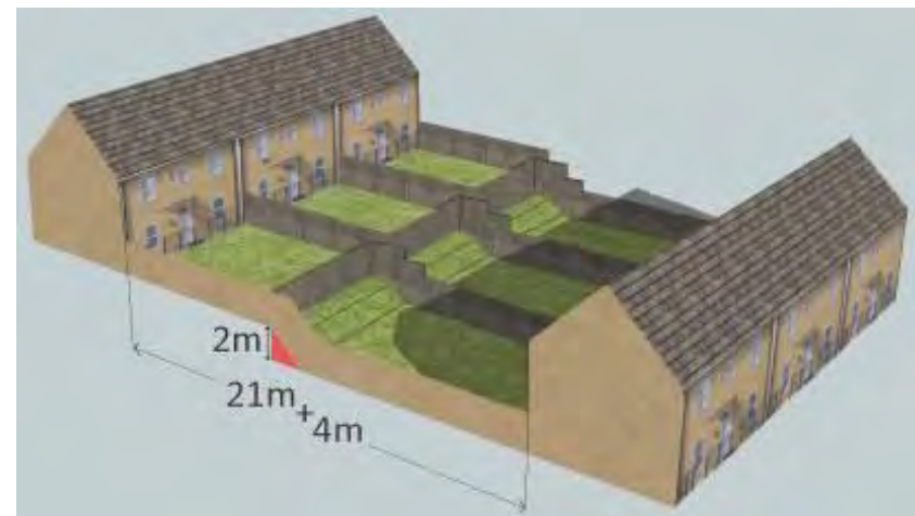
Fig K.10 Separation should be increased for homes at different levels
