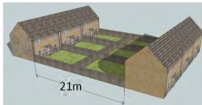
Fig K.8 The 21m separation distance is measured between rear elevations
