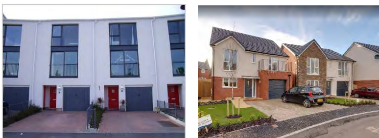
Fig L.5 Integral garages must not dominate frontages and should either be combined with living space at first floor above or in combination with habitable room windows at ground level.
