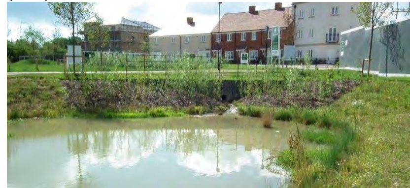
Fig E.4 SUDs features should be well integrated into open space areas as focal points (Source WWT online)
