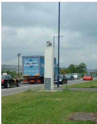
Photo 1 - St Thomas DOAS Transmitter
