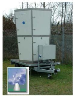
This equipment measures the wind speed and wind direction in 15m "layers" up to its maximum height range of 300m.
