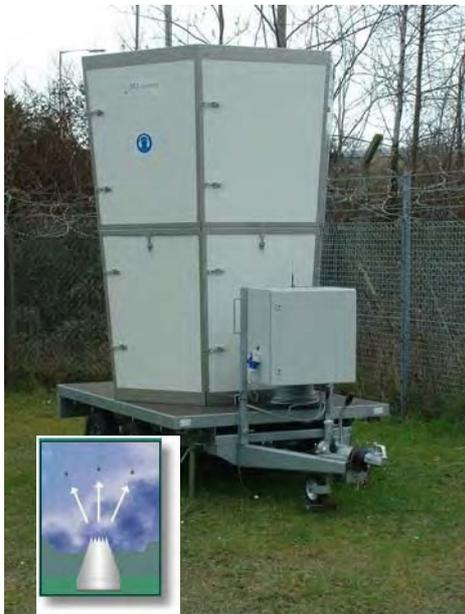
This equipment measures the wind speed and wind direction in 15m “layers” up to its maximum height range of 300m.
