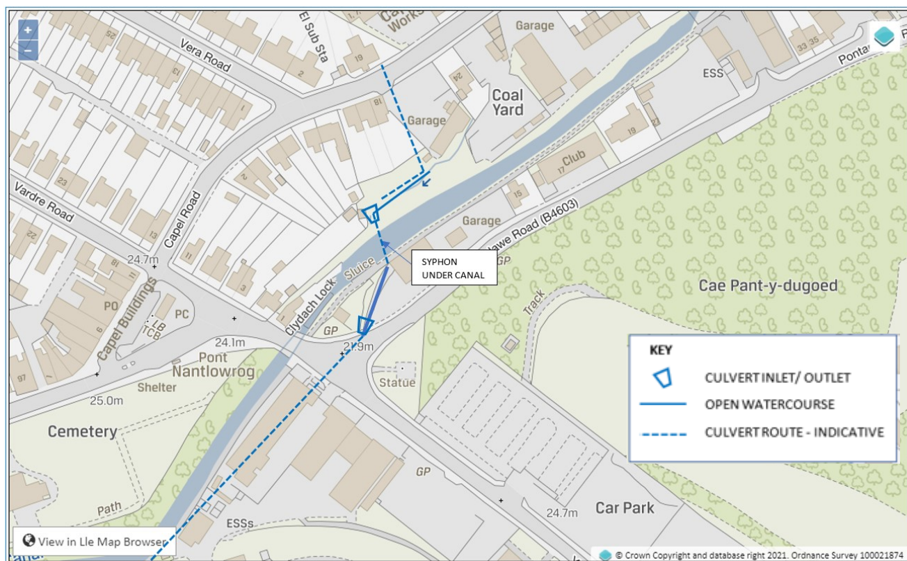
Figure 3-7 – Route of Enid Stream south of Capel Road via a syphon to the Canal outfall.
